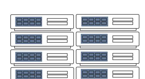
Lithium-ion batteries store energy ready to be supplied when needed. These are stacked on top of each other to form a battery rack and are connected together to reach the required voltage and current of the BESS. These are a tried and tested technology that is commonly used in our day-to-day lives, such as in smartphones.
