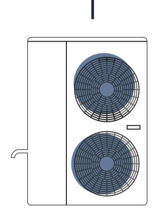
A heating, ventilation and air conditioning system controls the operating temperature within the system's enclosure and ensures good air distribution. This prevents the batteries from overheating, which in turn means that the batteries last longer and perform better.
