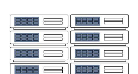
Lithium Iron Phosphate batteries store energy ready to be supplied when needed. These are stacked on top of each other to form a battery rack and are connected together to reach the required voltage and current of the BESS. These are a tried and tested technology that is commonly used in our day-to-day lives, such as in smartphones.
