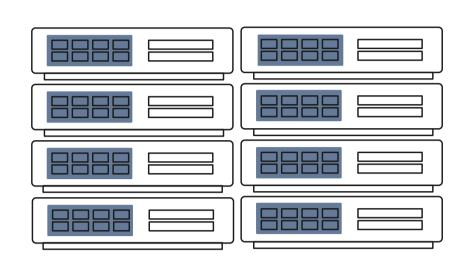
to be supplied when needed. These are stacked on top of each other to form a battery rack and are connected together to reach the required voltage and current of the BESS. These are a tried and tested technology that is commonly used in our day-to-day lives, such as in smartphones.
